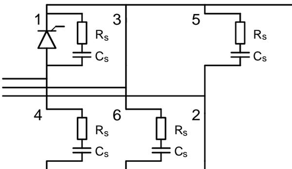
Fig. 9: Equivalent circuit when Thyristor 1 turns off
