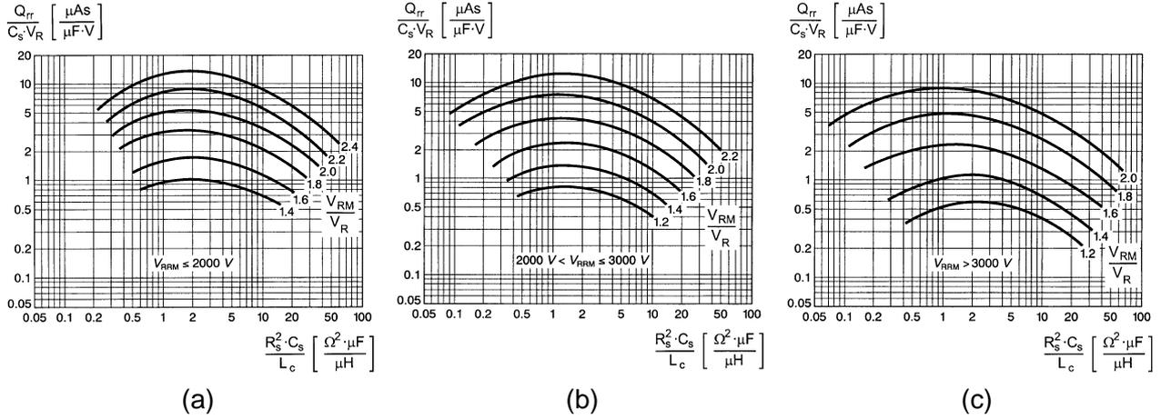
Fig. 7: Curves for determining the optimum RC snubber values of ABB phase control thyristors. The curves are valid for thyristors with  $V_{RRM}$  ratings below 2000 V (a), between 2000 and 3000 V (b) and above 3000 V (c). For diodes, similar curves apply but they depend somewhat more on the specifics of the design of the individual part number.
