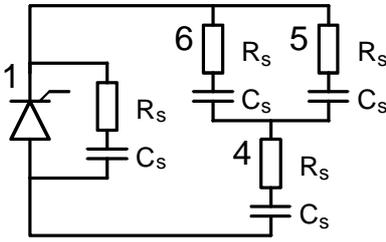
Fig. 10: Simplified equivalent circuit during turn-off of Thyristor 1
