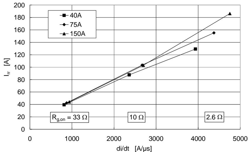
Fig. 7: Height  $I_{tr}$  of the reverse current peak versus  $di/dt$  at different currents ( $V_{DC} = 600V$ ,  $T = 125^{\circ}C$ ,  $L_{\sigma} = 50nH$ ).
