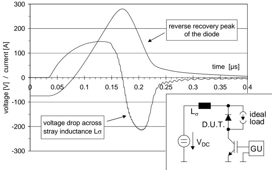
Fig. 2: Simulated switching characteristics of a diode, irradiated only with electrons ( $I = 75\text{A}$ ,  $V_{DC} = 600\text{V}$ ,  $di/dt = 5.4\text{kA}/\mu\text{s}$ ,  $L_{\sigma} = 40\text{nH}$ ). The voltage drop across the stray inductance  $L_{\sigma}$  proportional to the time derivative of the diode current.
