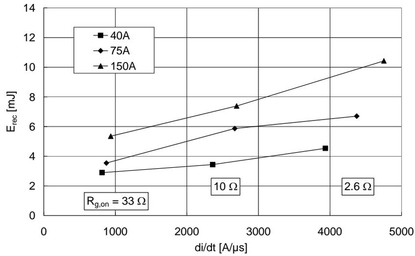
Fig. 9: Switching losses  $E_{rec}$  versus  $di/dt$  at different currents ( $V_{DC} = 600\text{V}$ ,  $T = 125^\circ\text{C}$ ,  $L_\sigma = 50\text{nH}$ ).
