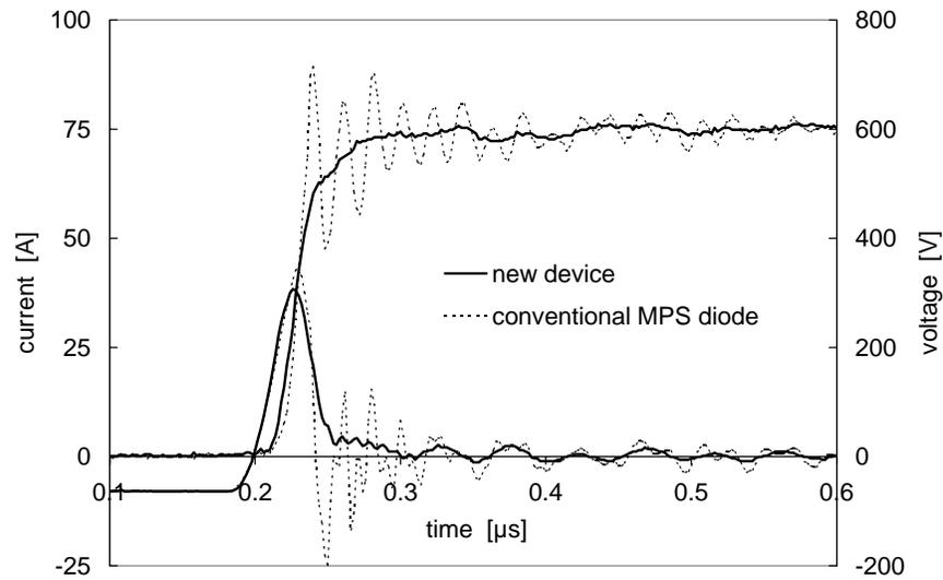
Fig. 6: Switching characteristics of the new diode and a conventional MPS diode at low current ( $8A \approx 0.1 \cdot I_{nom}$ ), room temperature (25°C), and medium gate resistor of 10Ω ( $V_{DC} = 600V, L_{\sigma} = 50nH$ ).
