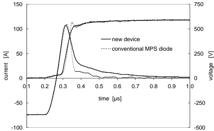
Fig. 5: Switching characteristics of the new diode and a conventional MPS diode at nominal current (75A), high temperature (125°C), and medium gate resistor of 10Ω ( $V_{DC} = 600V, L_{\sigma} = 50nH$ ).
