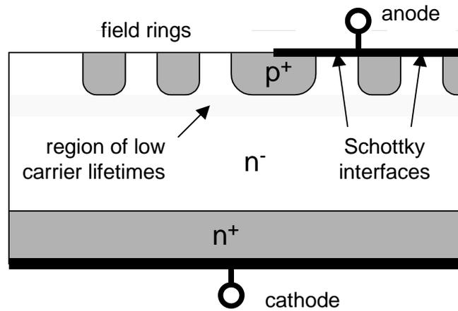
Fig. 1: Schematic of the new alpha irradiated MPS diode.
