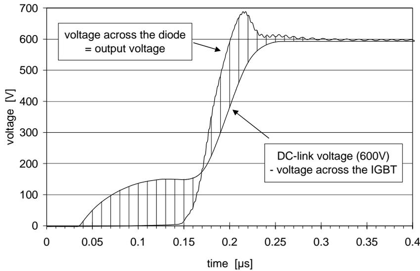
Fig. 3: Voltage across the diode (equals output voltage), and DC-link voltage minus voltage across the IGBT during the reverse recovery shown in Fig. 2. The shaded area represents the voltage across the stray inductance  $L_{\sigma}$ .
