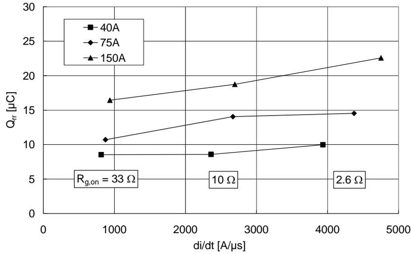
Fig. 8: Extracted charge  $Q_{rr}$  versus  $di/dt$  at different currents ( $V_{DC} = 600\text{V}$ ,  $T = 125^\circ\text{C}$ ,  $L_\sigma = 50\text{nH}$ ).
