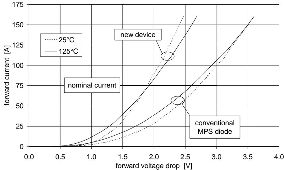
Fig. 4: Forward voltage drop of the new diode and a conventional MPS diode both measured at 25°C and 125°C
