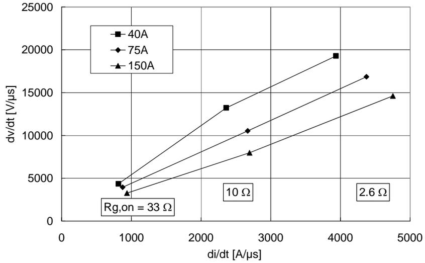
Fig. 10: Maximum dv/dt versus di/dt at different currents ( $V_{DC} = 600V$ ,  $T = 125^{\circ}C$ ,  $L_{\sigma} = 50nH$ ).
