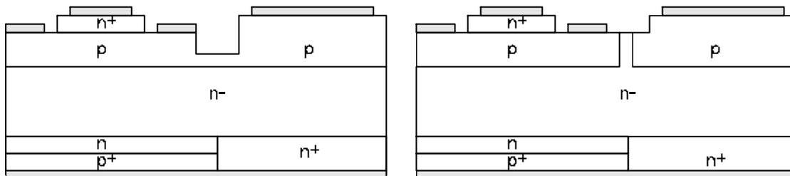
Figure 3: Comparison of resistive separation with npn separation of a GTO and integrated freewheeling diode. The advantages of the npn separation are very low gate leakage currents,  $I_{GRM}$ , and high blocking stability.
