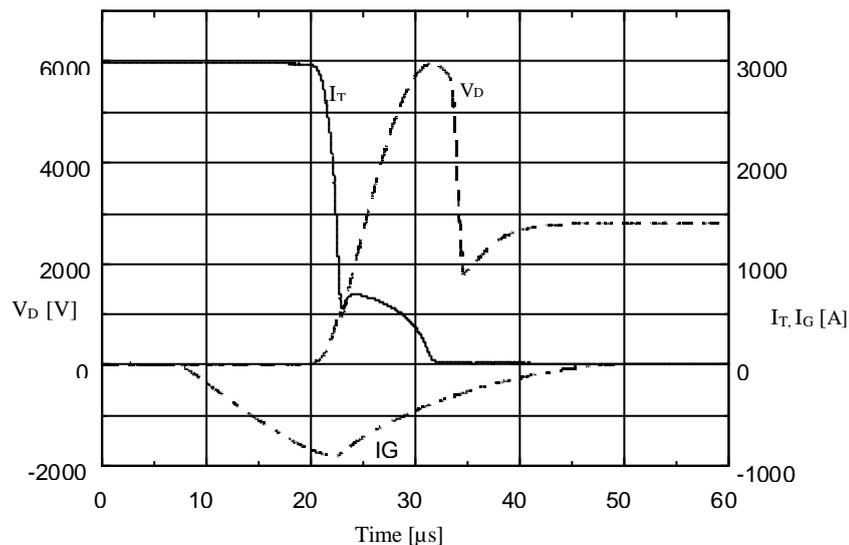
Figure 7: Turn-off waveforms of a 6 kV buffer layer GTO. The on-state of this device is 3.25 V at 3 kA and 110 °C. The turn-off conditions are  $C_s = 2.66 \mu\text{F}$ ,  $L_s \approx 250 \text{ nH}$   $di_g/dt = 70 \text{ A}/\mu\text{s}$ ,  $T = 110 \text{ }^\circ\text{C}$ .
